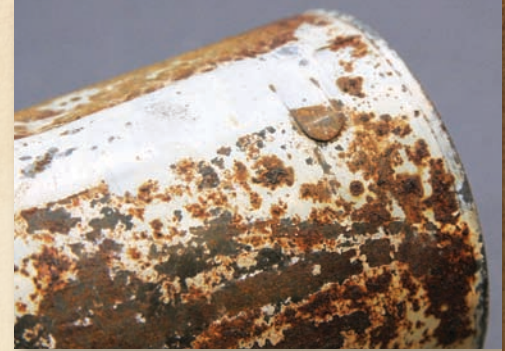
TAB FOR KEY WIND OPENER ON MACHINE SOLDERED CAN PICTURED AT BELOW LEFT
