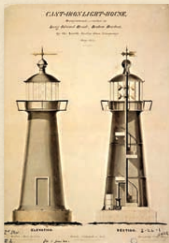
THE LONG ISLAND HEAD LIGHTHOUSE WAS AMERICA'S FIRST CAST IRON TOWER
