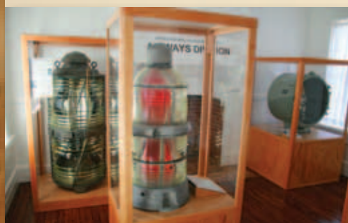
LIGHTHOUSES FOR AIRPLANES EXHIBIT AT THE PONCE DE LEON INLET LIGHTHOUSE. FROM LEFT TO RIGHT: SPERRY AGA LANDINGFIELD FLOOD LIGHT, FAA CODE BEACON, DCB-24
