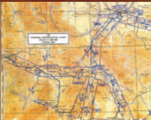
1943 PILOT'S SECTIONAL CHART SHOWING AIR ROUTE FROM BUTTE TO HELENA TO GREAT FALLS. BEACONS APPEAR AS SMALL STARS. THE ACCOMPANYING MORSE CODE SIGNALS ARE SHOWN NEAR EACH STAR. COURTESY OF MIKE ROGAN
