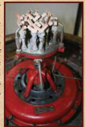
THE BEACON WAS ILLUMINATED WITH AN AGA SYSTEM DALEN 30-CLUSTER COMPLEX FLASHER ACETYLENE BURNER
