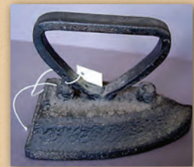
THE HANDLE OF THIS IRON COULD BECOME ALMOST AS HOT AS THE SOLE
