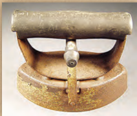
HOT COALS WERE PLACED INSIDE THIS IRON
