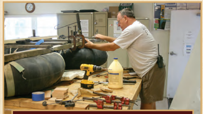
WHEN THE TIRES HAVE BEEN STABILIZED, THE FRAMEWORK IS REPAIRED.
