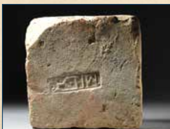
Unlike adobe, fired brick was strong, durable, and almost impervious to the effects of moisture, wind, and other natural factors that could cause deterioration. This Roman brick was made by the First Roman Legion.
