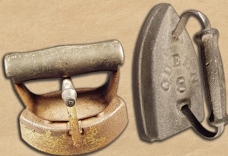
A SAD iron with a detachable wooden handle (left) and An eight-pound SAD iron with a metal handle (right); collection of the Ponce de Leon Inlet Lighthouse Preservation Association
